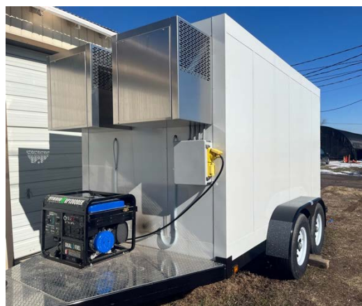
7'x12' refrigerated trailer (-18 °C ~ 10 °C)
