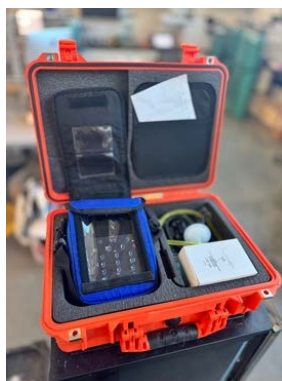
Biogas 5000 Portable Analyzer with H 2 S, H 2 , CH 4 , CO 2 , O 2 , temperature, and pressure probes
