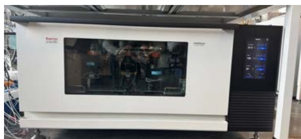
Thermo Scientific IntelliStack Incubator Shaker with a front down swing door and 690 x 1005 x 347 mm internal space
