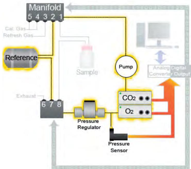
Gas Sensor Technologies: The Micro-Oxymax uses several types of gas sensor technologies to measure the concentrations of different gases. These include Paramagnetism, Electrochemical Fuel Cells, and Non-Dispersive Infrared detection. Following is a brief description of each and their principle of operation.
