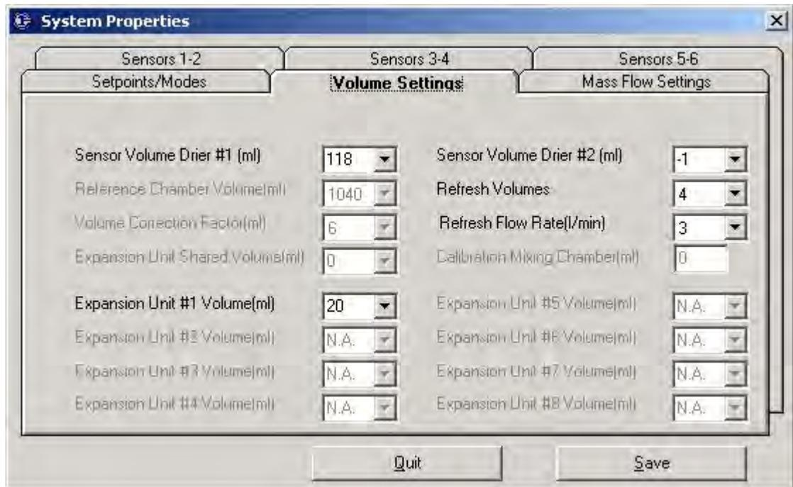
**Sensor Volume Drier 1 and Drier 2.** These volumes are used to set the internal sensor volume through drier 1 and drier 2. These volumes include all the internal volumes of the sensors, tubing and the drier itself. These volumes are automatically measured when ever the volume measurement utility is performed.
