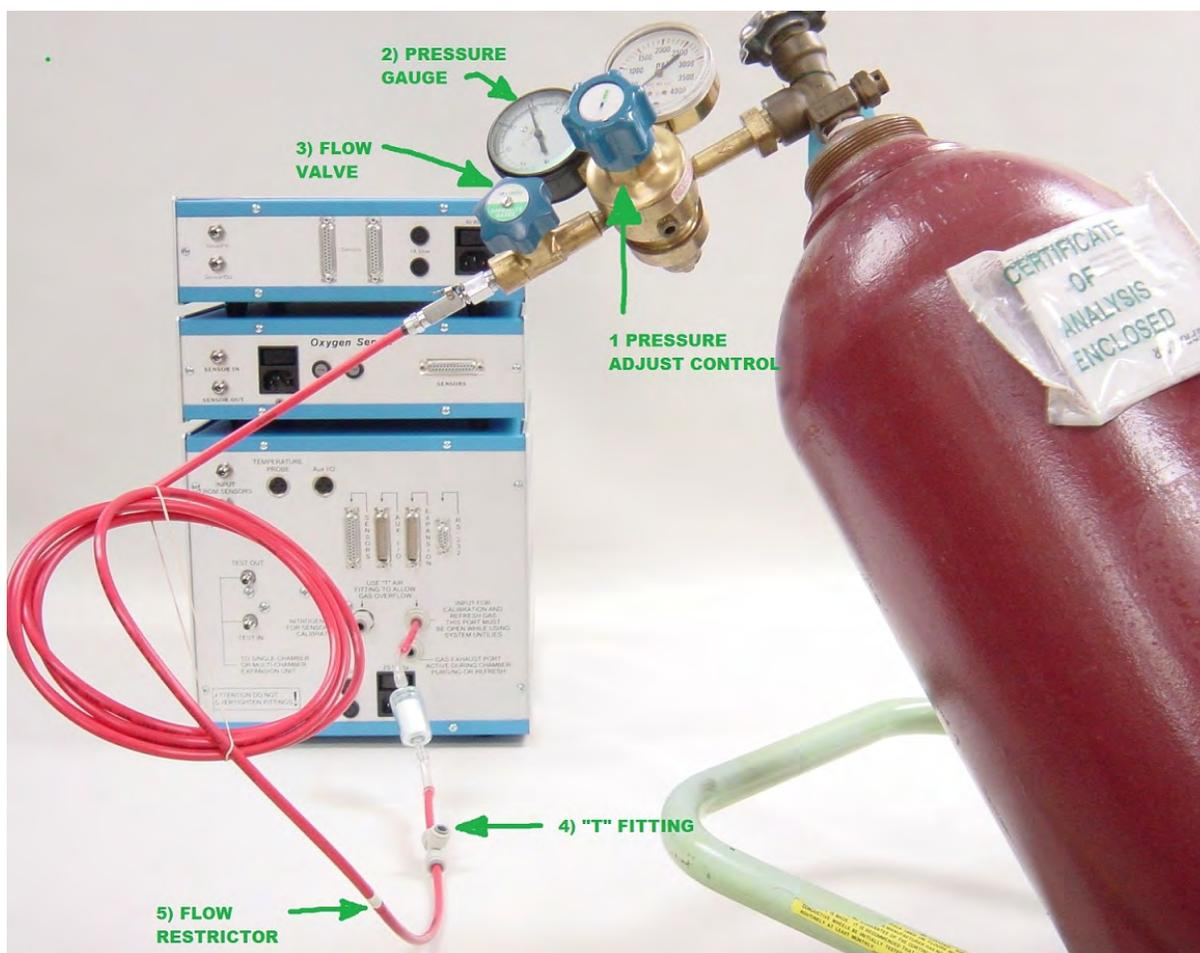
A dual stage pressure regulator must be connected to the cylinder. The pressure control knob (1) should be adjusted for a reading of 5 PSIG on the pressure gauge (2). Some regulators will have a flow control valve (shown as number 3 in the picture). Make sure this is opened fully counterclockwise to allow flow of gas.
