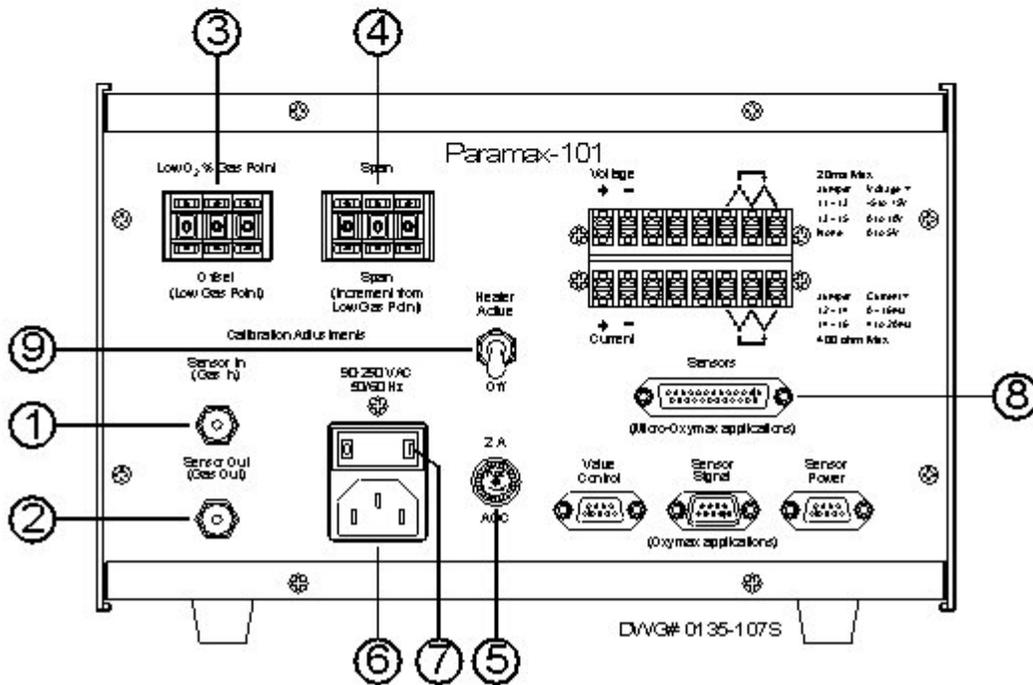
**1. SENSOR IN FITTING.** This is connected to the "Sensor Out" connector on the CO<sub>2</sub> sensor, or to the "Sensor Out" connector on the System Sample Pump for O<sub>2</sub> only systems.
