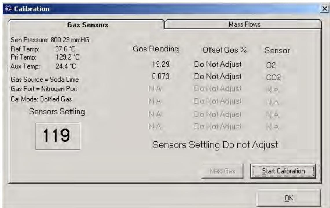
After the timer reaches zero, then the user will be prompted to adjust the zero knob on each sensor for a reading of 0 on the screen. The numbers will turn blue to indicate which sensor(s) should be adjusted at this point. The timer will start increasing after it reaches 0, just ignore this.
