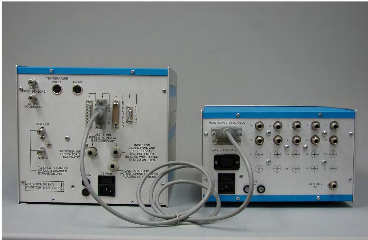
Connect the cable from the Aux I/O connector on the rear of the system sample pump to the mass flow meter out connector on the rear of the equal flow box. If there is more than one equal flow box is used connect the remaining mass flow meter signal out connector to then mass flow out connector of the next equal flow box
