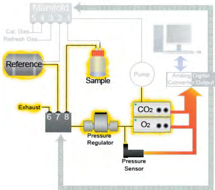
Step 2: Measuring the sensor volume is next. The sensor volume is important to know so that the volume can be accounted for and subtracted when the sample is measured. When the gas analyzers report their values, it includes gas concentrations inside the Sample Chamber plus all of the tubing and the sensors themselves. Since concentration is a percentage of a volume, the sensor and plumbing volumes must be subtracted to yield accurate measurements for the sample.
