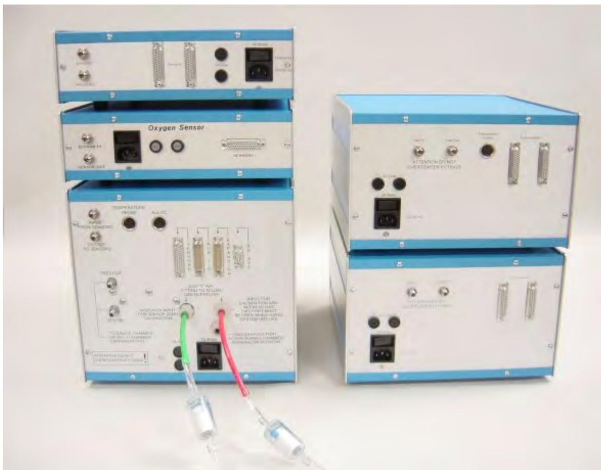
Connect the large drier filled with Soda Lime (white granules) as shown in the drawing. The bottom fitting (the sealed end) of the large drier connects to the fitting labeled "Nitrogen" on the back of the System Sample cabinet with 1/4" tubing. If the paramagnetic O<sub>2</sub> sensor is used there will not be a soda lime column, instead a line going to a tank of offset gas will be connected to the N<sub>2</sub> port (see calibration section of the manual)
