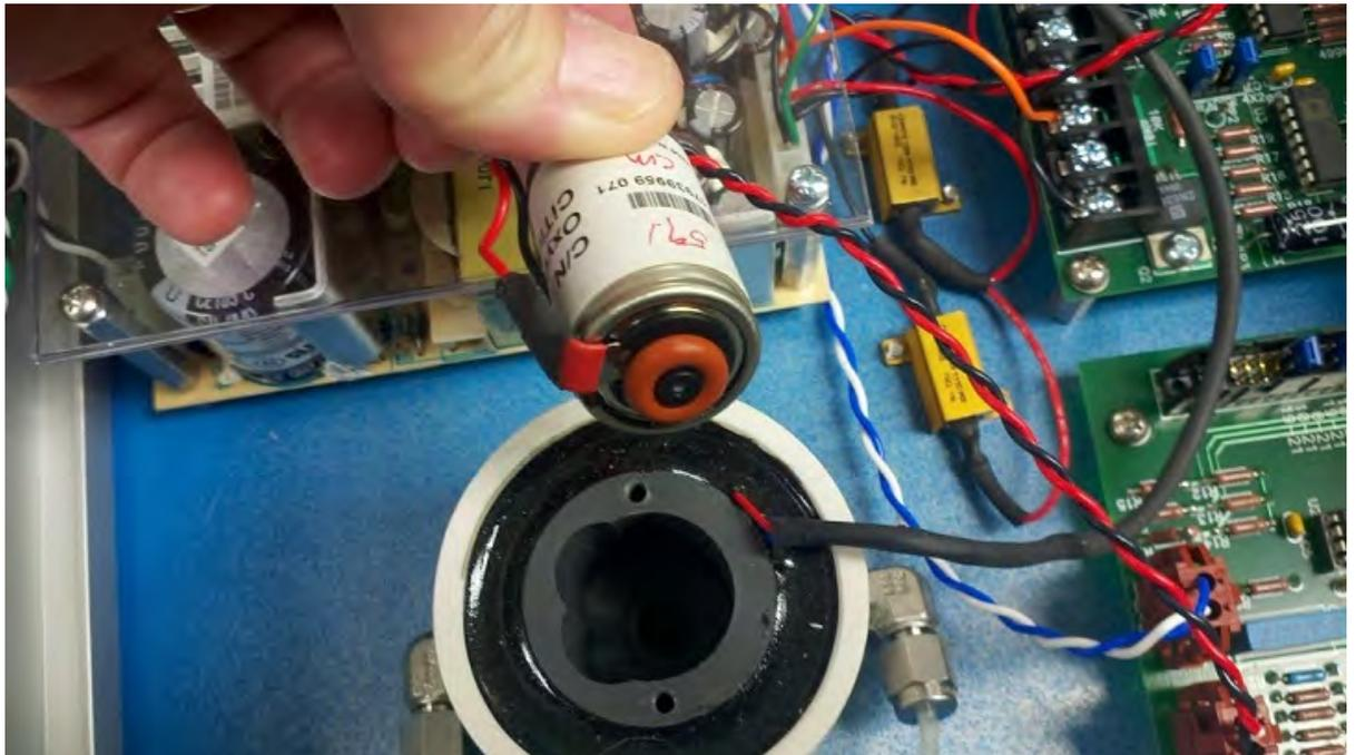
11. Replace the cover over the sensor cell making sure the relief slot for the wires is positioned over the place where the wires come out of the housing
