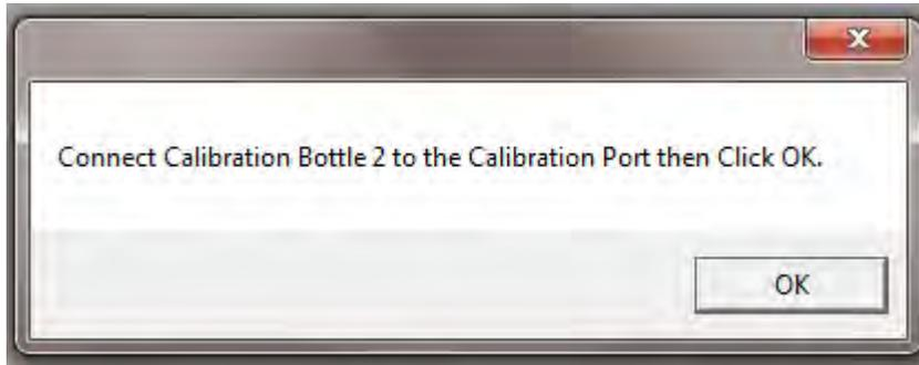
Again the screen will start counting down to zero and then will prompt to adjust the span on the sensor colored in blue so the values in the gas reading column are equal to the values in the Span gas % column.
