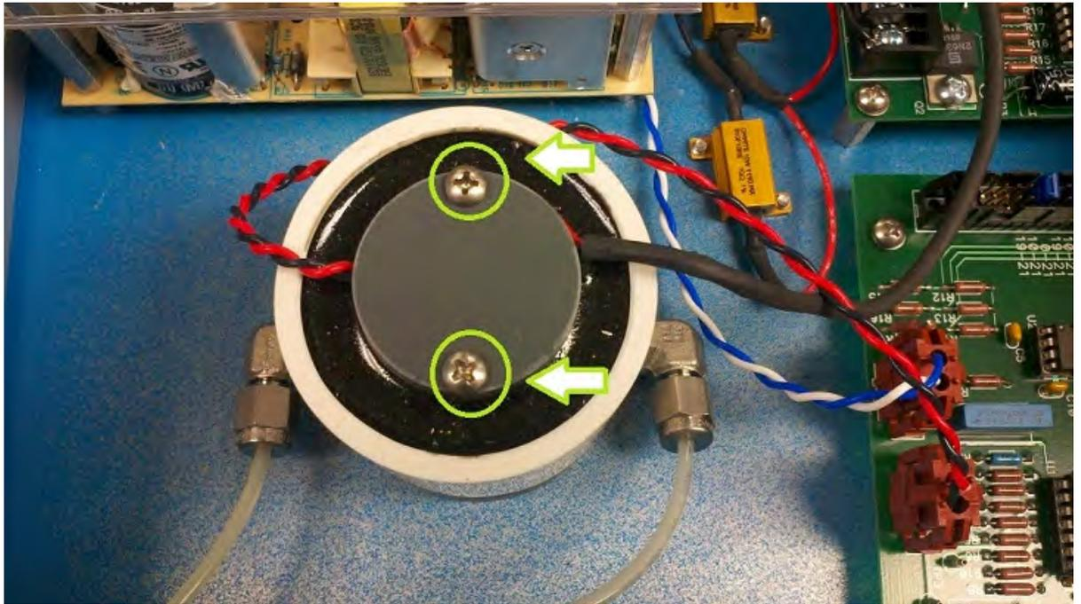
8. Slide the sensor assembly out and remove the red and black wires from the plug in connector on the circuit board
