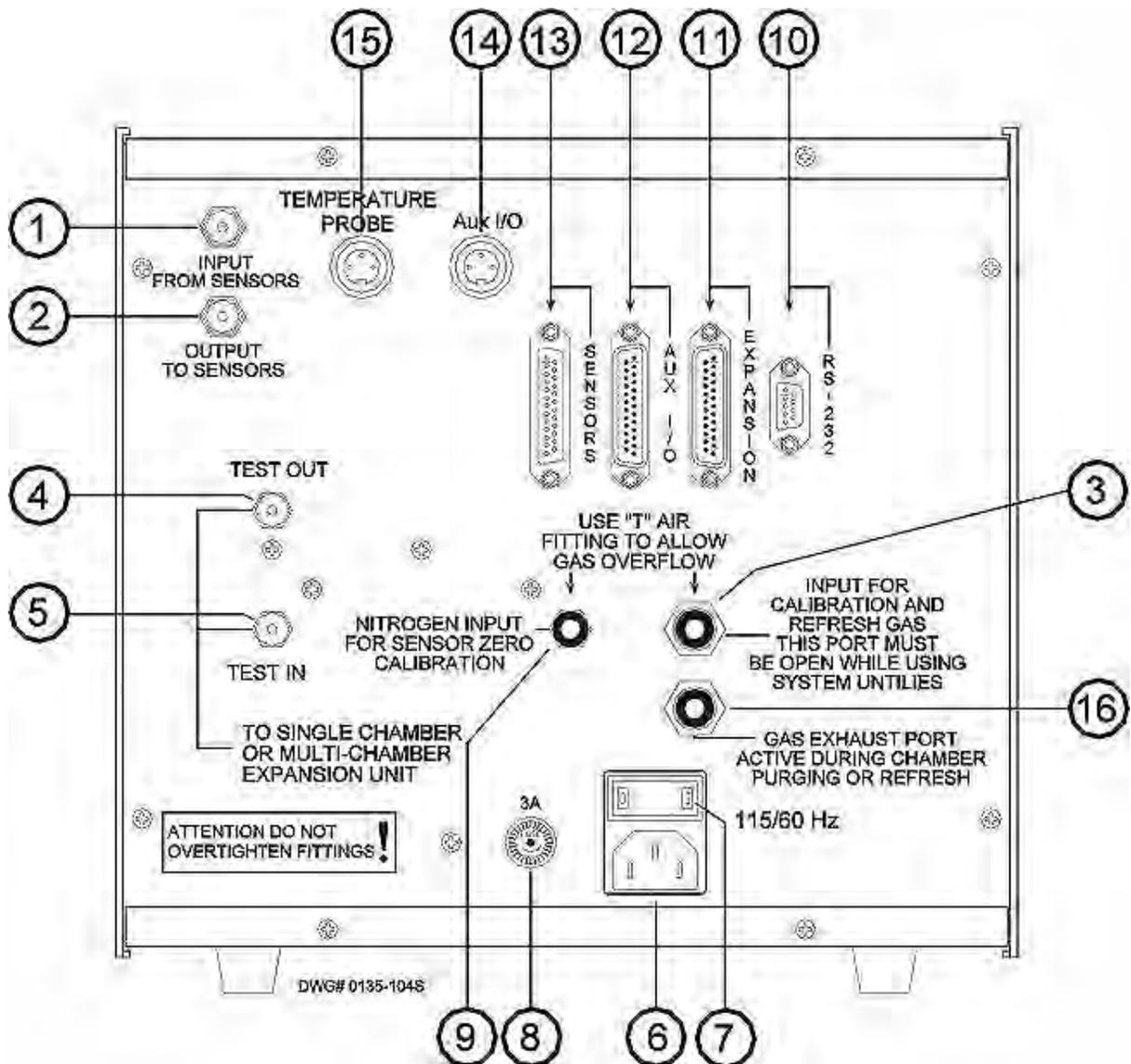
**1. SENSOR IN FITTING.** This is connected to the "sensor out" connector on the O<sub>2</sub> sensor.
