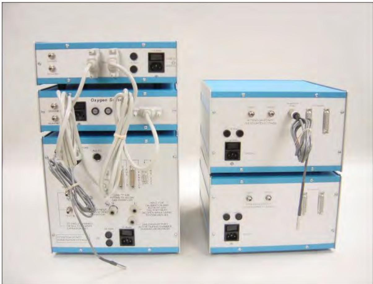
Each additional sensor is connected in series with the 25 pin cables
