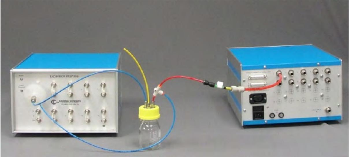
This is the configuration where the fresh air flow is less than the ample flow and the sample air is recirculated to the measuring chamber. So there will be a tube connected from the test out port back to the chamber.
