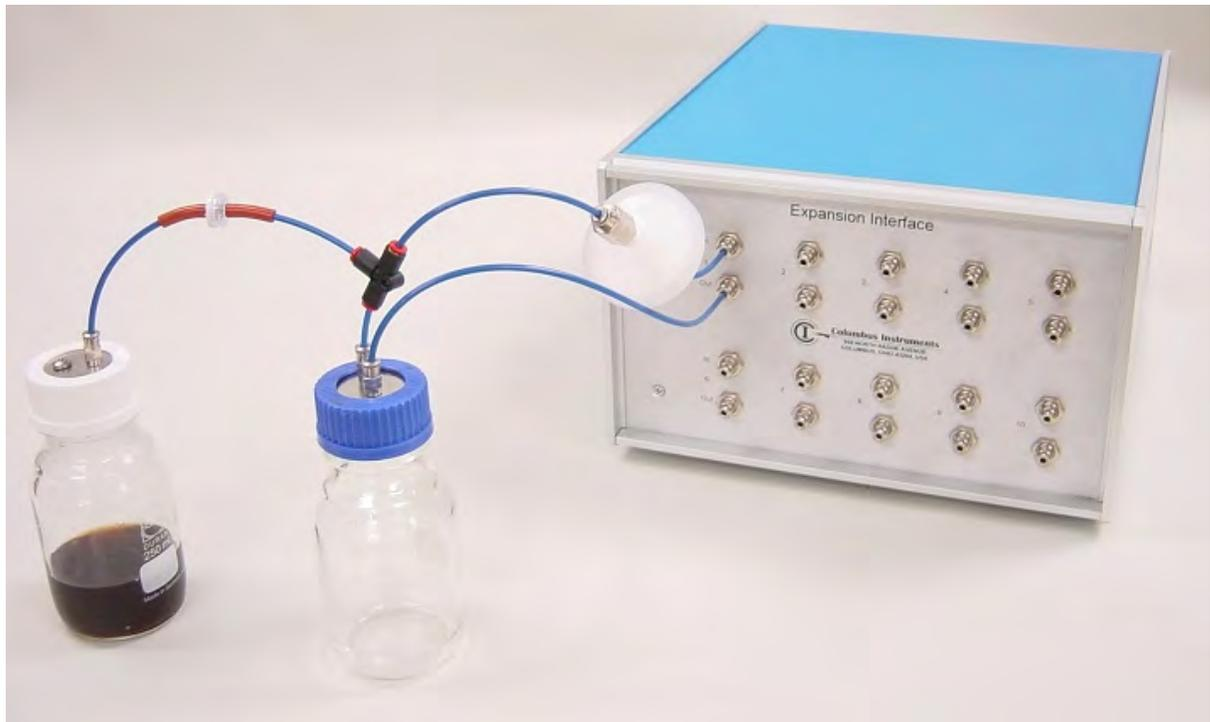
Be sure the clear side of the one way valve points to the sample bottle:
