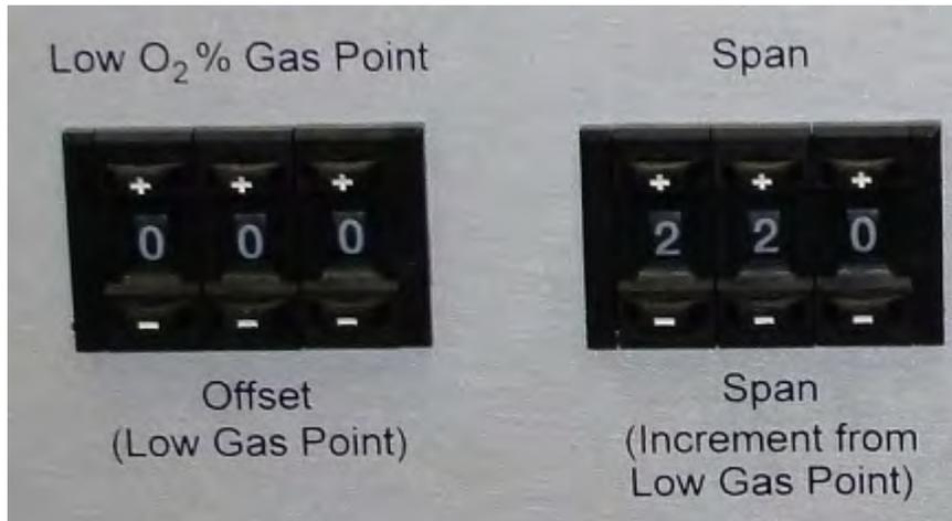
In the below example the range of the sensor will be 19 - 21% O<sub>2</sub>. An offset gas with 19% O<sub>2</sub> will be required as well as a span gas with 90% of the full range would be required. (actually ambient air can be used, it contains 20.93% O<sub>2</sub>)
