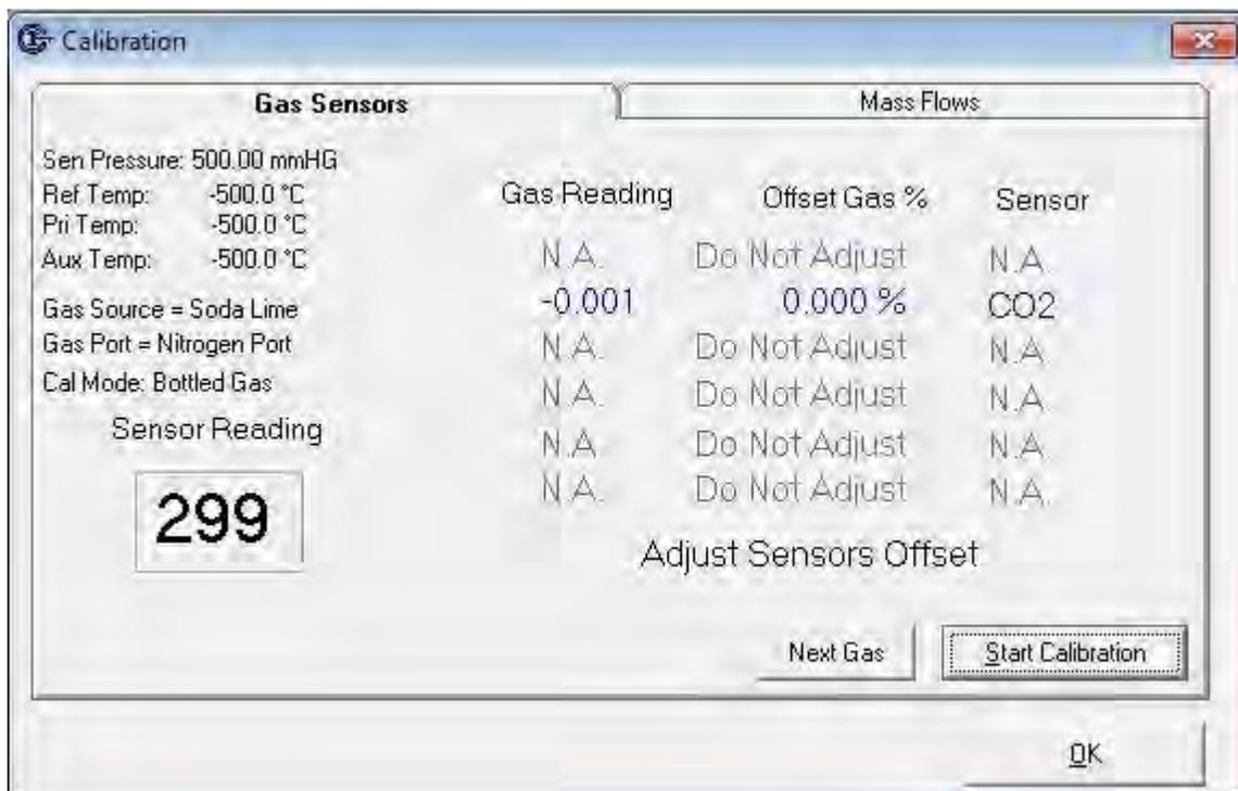
After the knob(s) has been adjusted, click on the button labeled "next gas" The software will then prompt you to connect the calibration cylinder to the calibration port. Ensure the bottle is connected as shown previously in this section then click ok.
