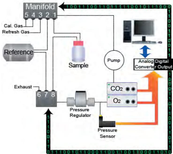
**Reference Chamber:** This is exactly 1L in volume and made of stainless steel. It has two main functions. 1) It is a fixed volume that we use to calculate sensor and sample head space volume using various pressures. 2) It stores a known concentration of air that we use to calculate sensor drift after each measurement cycle.
