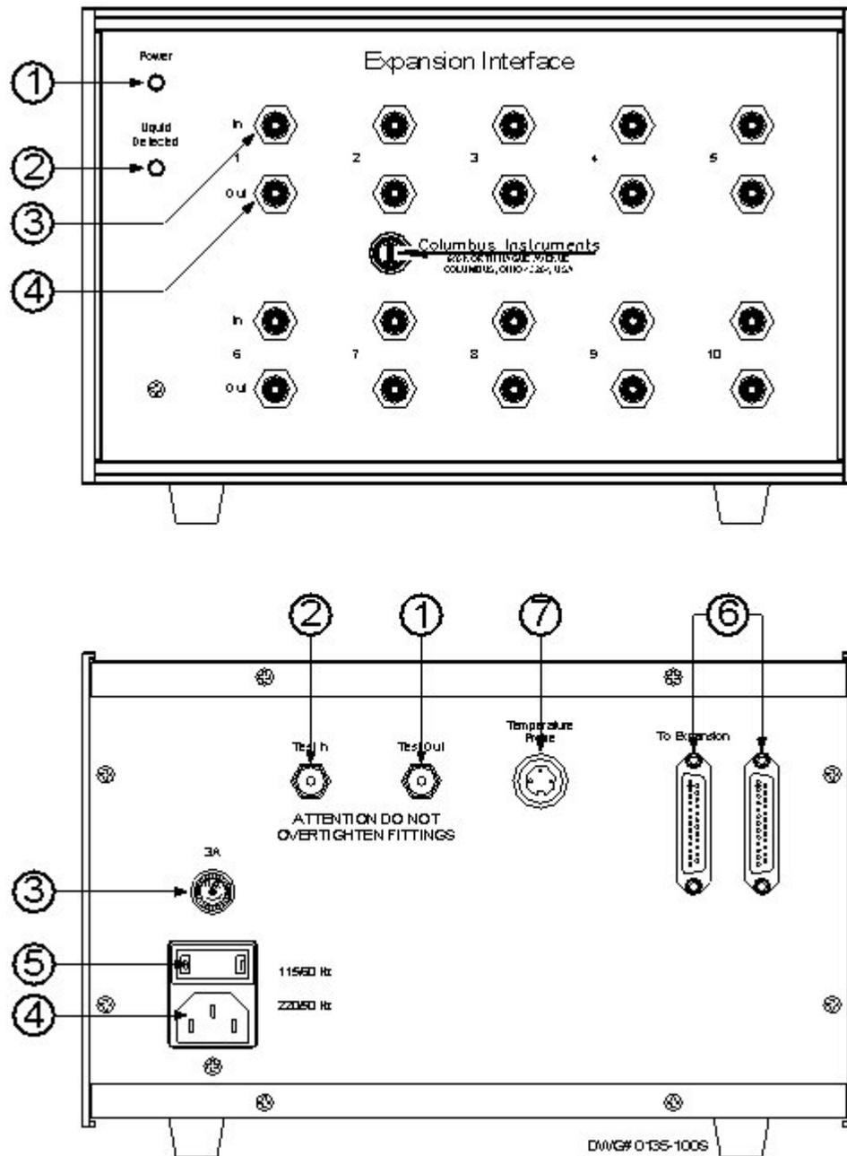
1. **TEST OUT FITTING.** This is connected to the "Test In" fitting on the Sample Pump.
