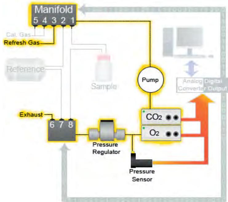
Step 7: We can finally measure our sample! The System circulates the gases from the head space of the Sample Chamber through the sensors then re-circulates them back into the Sample Chamber for a factory set time period of three minutes, and takes a reading from the sensors.
