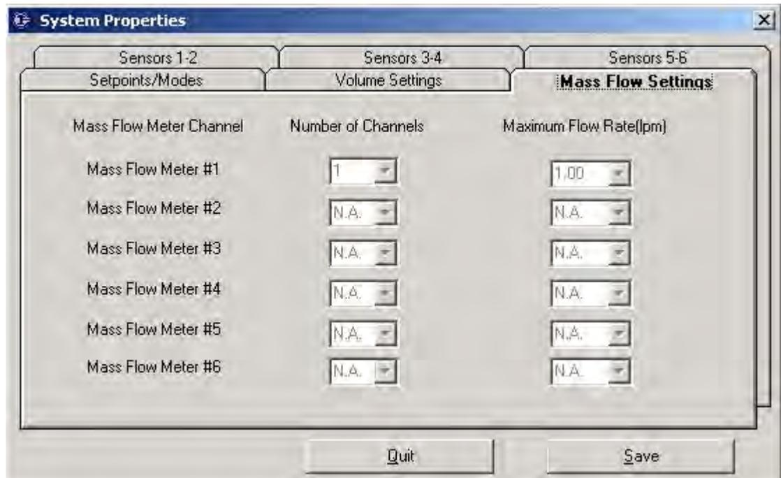
**Mass Flow Meter 1-6**. The Micro Oxymax is capable of running with 6 different mass flow meters. Each mass flow meter can have one or more channels associated with it. In the case of
