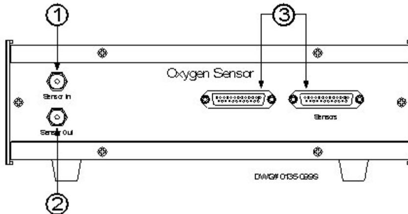
1. **SENSOR IN FITTING.** This is connected to the "Sensor Out" connector on the CO<sub>2</sub> sensor, or to the "Sensor Out" connector on the System Sample Pump for O<sub>2</sub> only systems.
