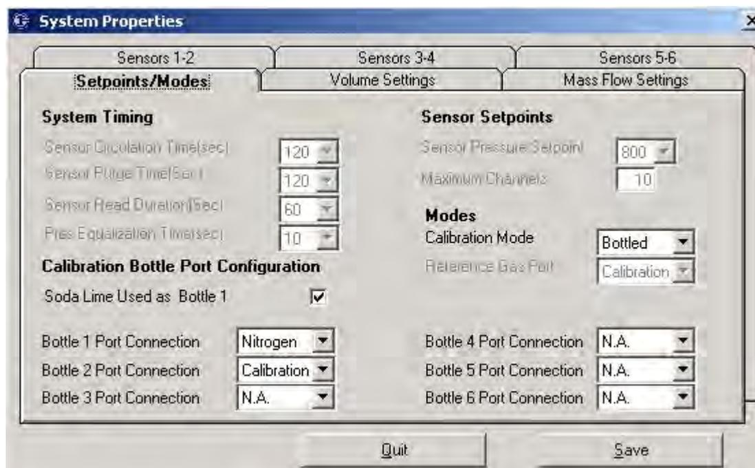
**System Timing.** These values are used to set the amount of time the system circulates gases during purging, settling and purging of the system. These values are factory set and can not be changed.
