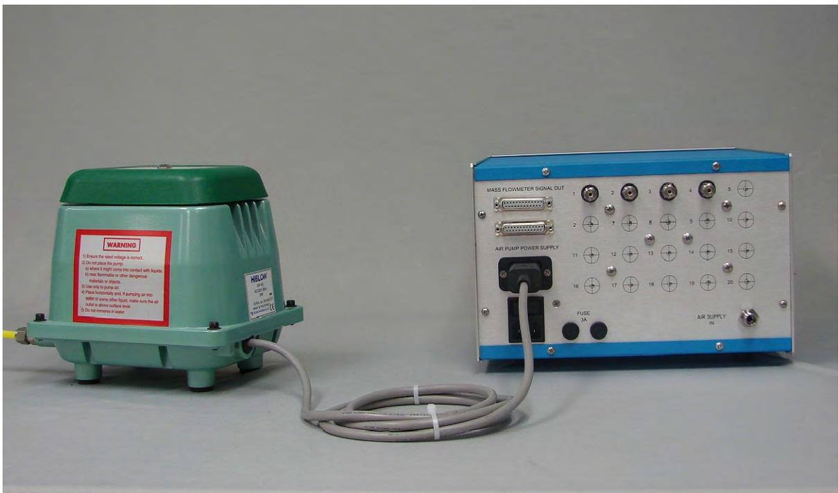
Connect the electric power cable from the fresh air supply pump to the air pump power supply connector on the rear of the equal flow air supply system
