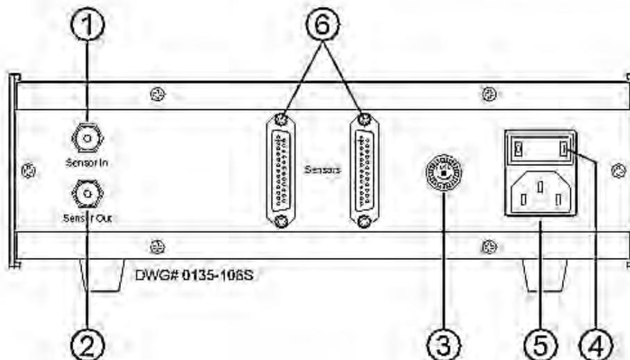
**1. SENSOR IN FITTING.** Connects to the Sensor Out connector on the System Sample Pump.
