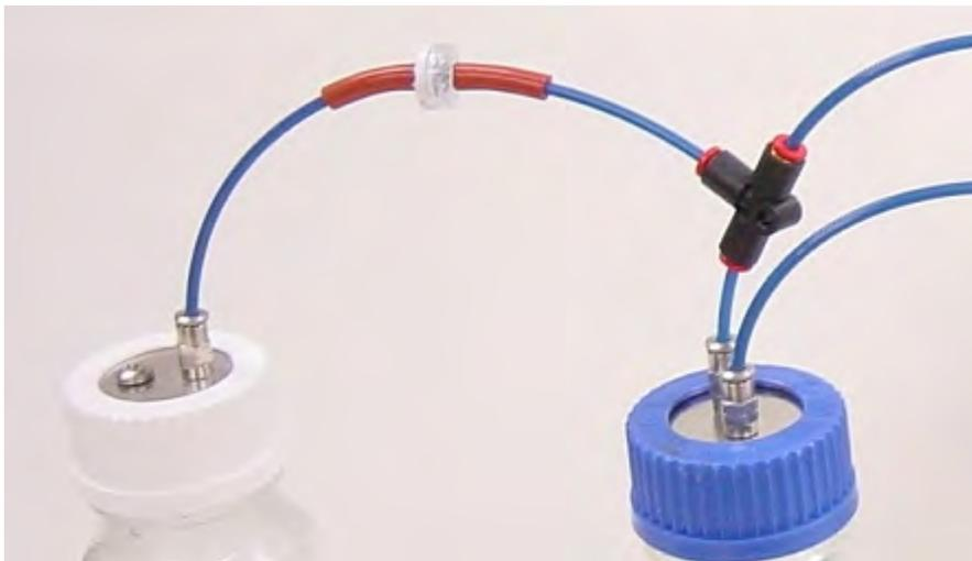
Connection with the condenser with a 3 port flask
