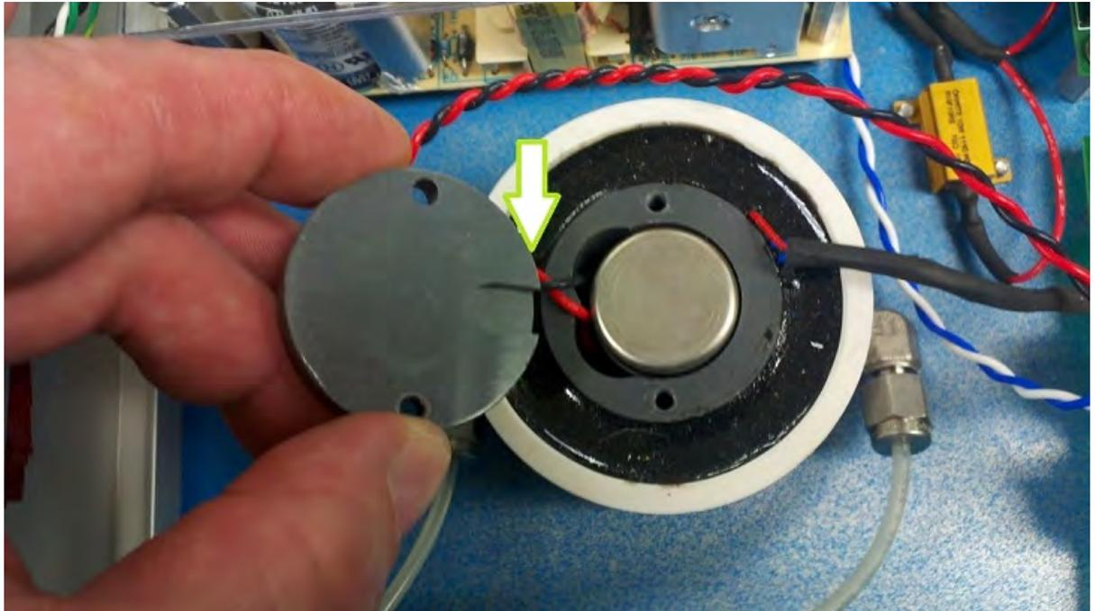
12. Replace the top panel and secure it with the two Philip's screws and lock washers.
