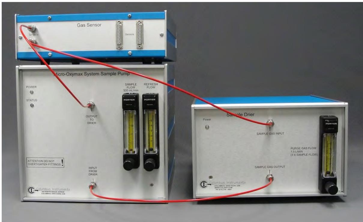
If any additional toxic gas sensors are used they should be connected in series as below
