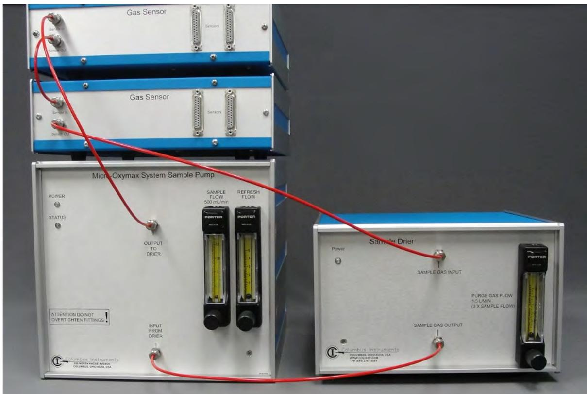
If the system does not include an Expansion Interface (for a single channel system), connect the test chamber directly to the System Sample Pump. Cut two pieces of tubing long enough to reach from the test chamber to the System Sample Pump. These are used to connect the test chamber to the "Test In" and "Test Out" fittings on the back of the System Sample Pump.
