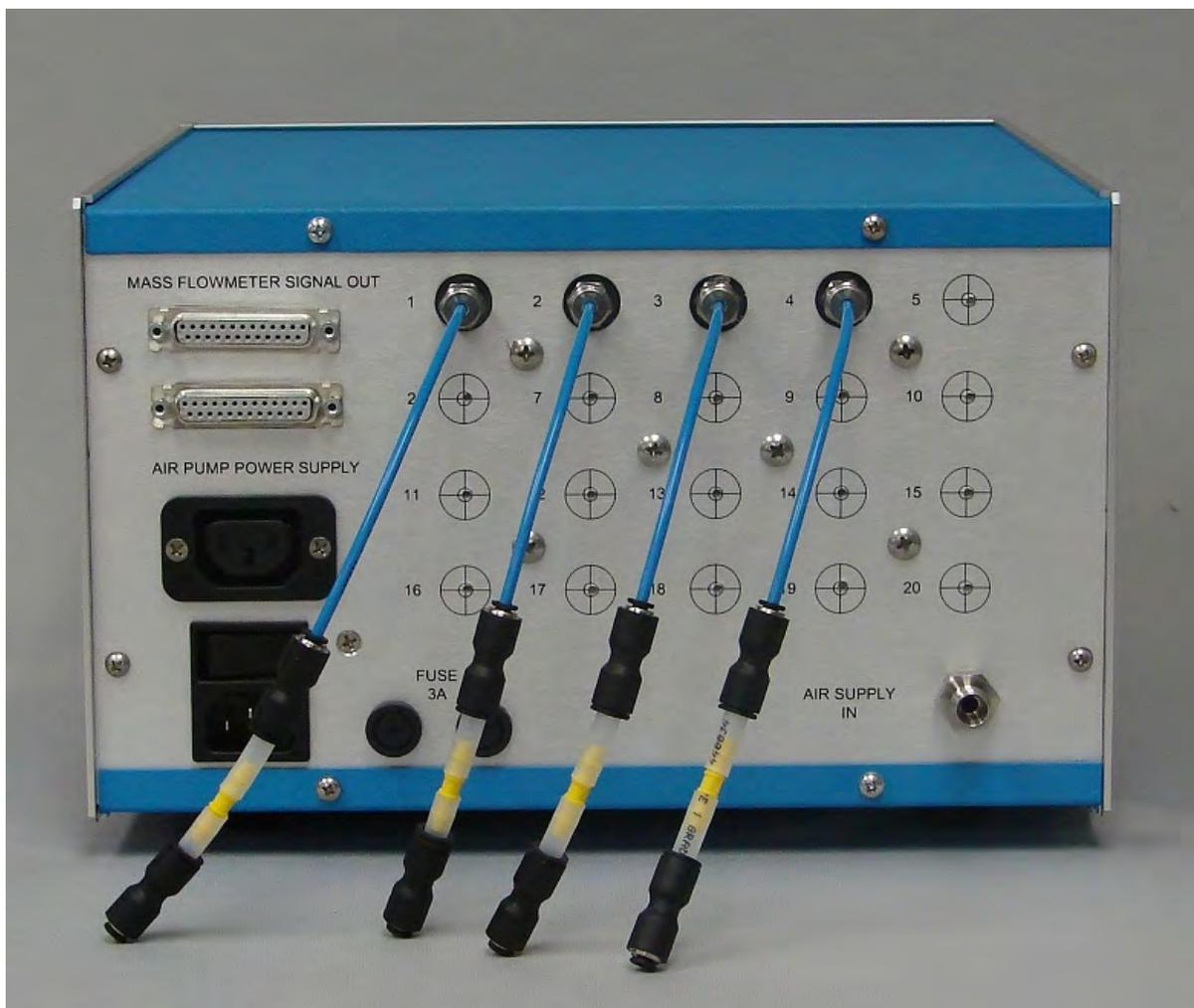
Connect the flow restrictors as shown for all channels. Please note all ports must have the restrictors connected even if all channels are not being used!
