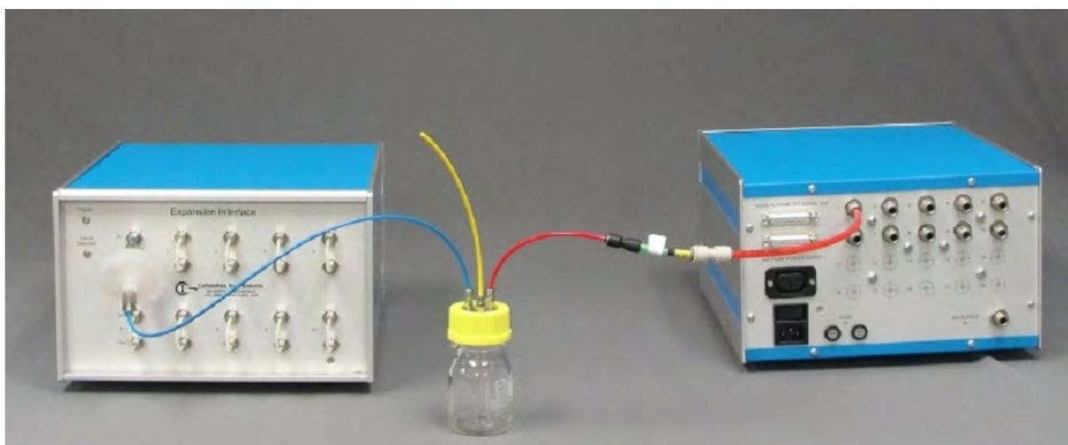
Now connect the tubes from test in port on the expansion interface to the sample chamber. This is the standard connection used when the fresh air supply flow is greater than the sample flow and the out port from the expansion interface is exhausted to the atmosphere and not recirculated to the chamber. Note the yellow tube for the extra overflow air to come out.
