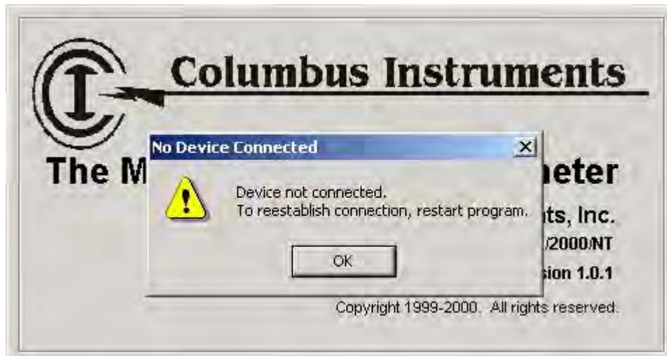
As the software loads the system will automatically search the computers communication ports for the Micro Oxymax hardware. If the hardware is not found then the user will be notified that the Device is not connected. The program will need to be restarted to reestablish the connection with the hardware.
