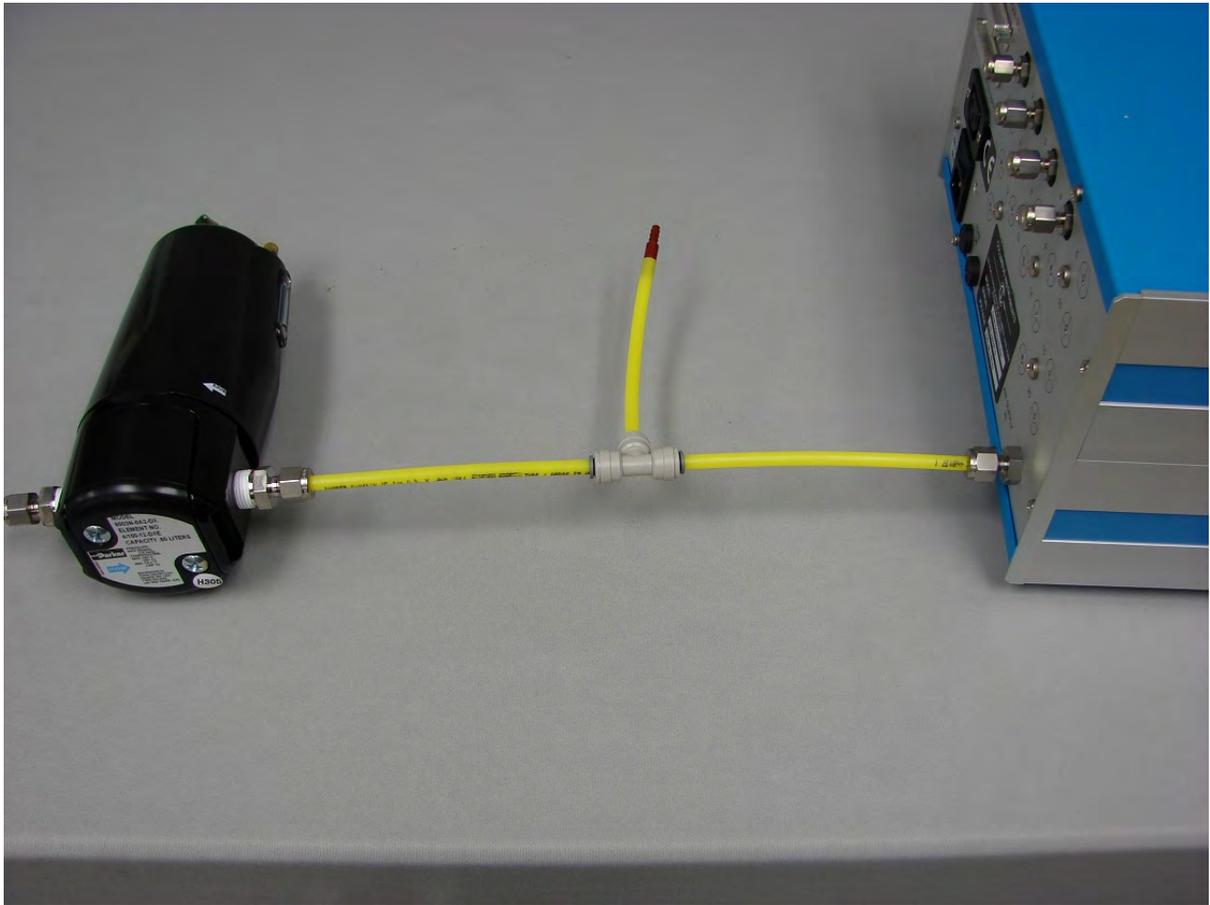
Connect the fresh air pump to the filter then connect the filter to the air supply in connector on the rear of the equal flow box. Note that the arrow on the filter should point towards the equal flow box, or if the filter is marked with in and out the pump must be connected to the in port.
