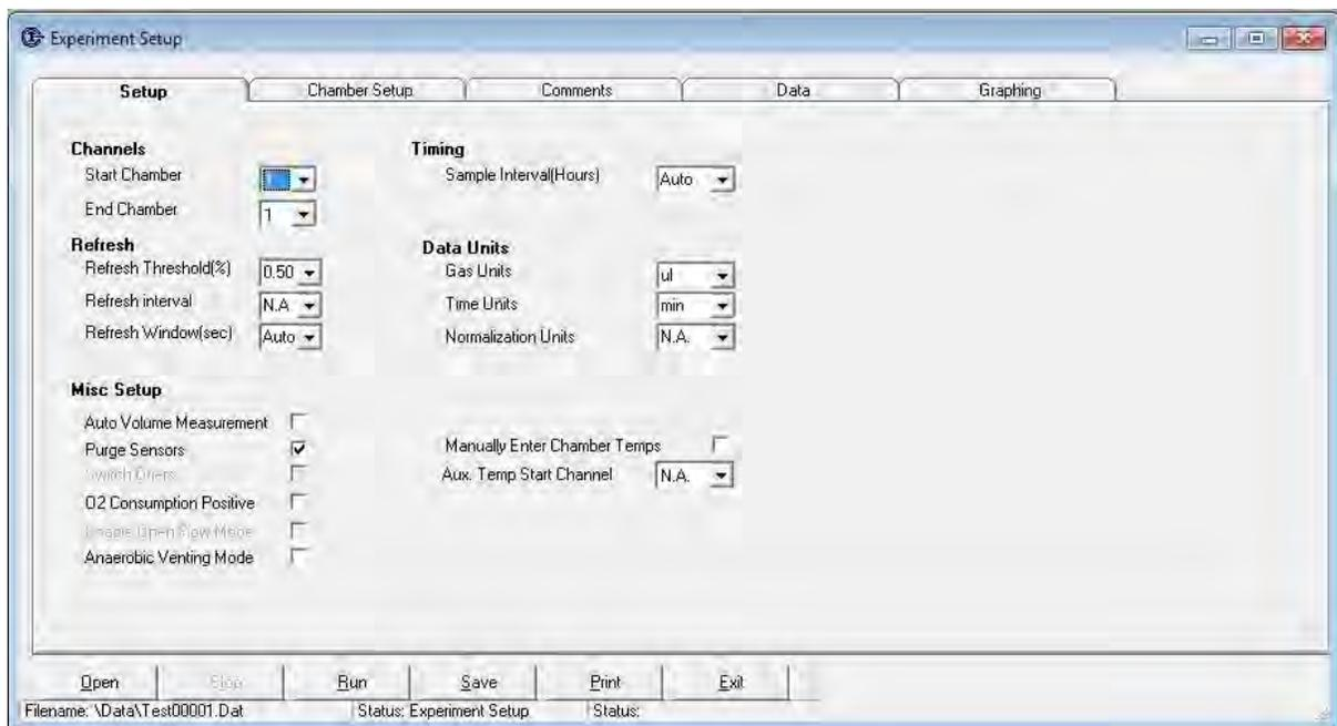
**Start Chamber and End Chamber.** Any contiguous group of chambers can be selected for an experiment. The Start chamber is the smallest numbered chamber, the End chamber is the largest numbered chamber. The experiment will read from the Start chamber through the End chamber inclusive. An experiment with only one chamber has the End chamber number = Start chamber number.
