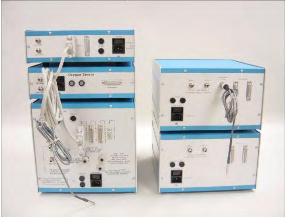
The second cable should connect the first sensor to the second sensor, and so on until all the sensors are connected together.
