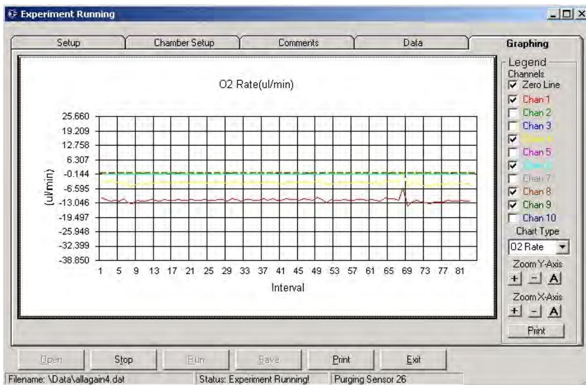
**Channel Selection.** When graphing experiment data, a total of ten chambers can be displayed at one time. If an experiment contains more than ten chambers any chamber can be displayed at one time, however the total chamber displayed at one time is limited to ten. A Zero line can be displayed to show the zero line on the graph. The Zero line is displayed as a black dashed line.
