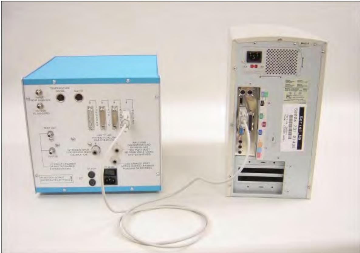
Use the remaining 25 pin cables with male connectors to connect the expansion units to the system sample pump. Like the sensor cables, there will be one cable per expansion unit. The first expansion unit is connected directly to the system sample pump's connector labeled "Expansion Unit". Additional expansion units are connected in series to one another through the additional 25-pin cables.
