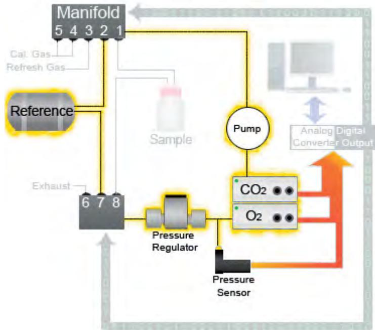
Step 6: Now the purge gas concentrations are measured. This step is rather important. In between the measurement of each sample, the sensors are purged with ambient air to remove the residual gas left in the sensors from the previous sample. But when we measure the next sample, the small amount of gas inside the sensors is mixed with the Sample Chamber gas. So the purge gas is measured by the gas sensors so we know what we've mixed in. We later subtract it from the sample's measurement.
