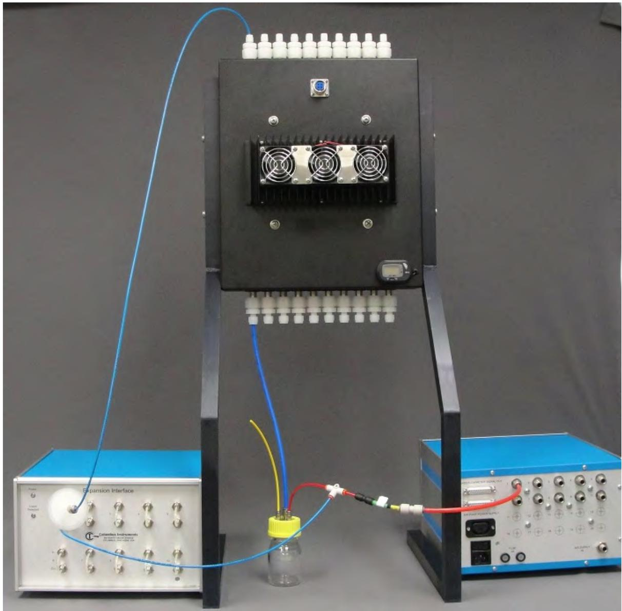
The connections for the open flow option with the condenser are shown. This is for the configuration where the fresh air flow is less than the sample flow and the sampled gas is recirculated back to the chamber
