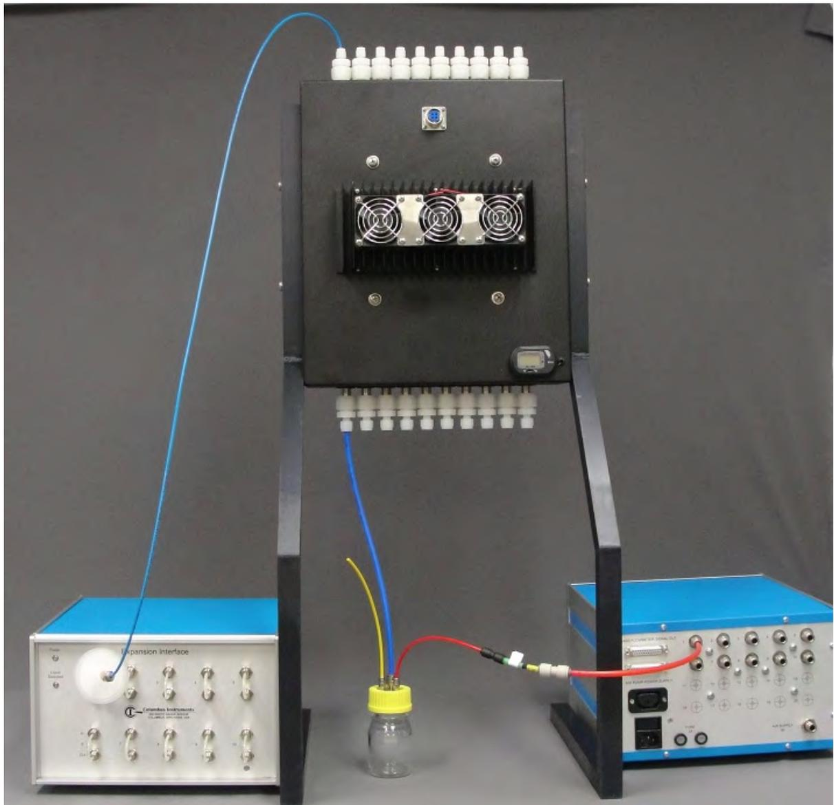
if a condensing air drier is used the connection will be slightly different as shown below (the main difference being the additional tube coming from the condenser to the bottle. This is the configuration where the fresh air flow is greater than the sample flow.
