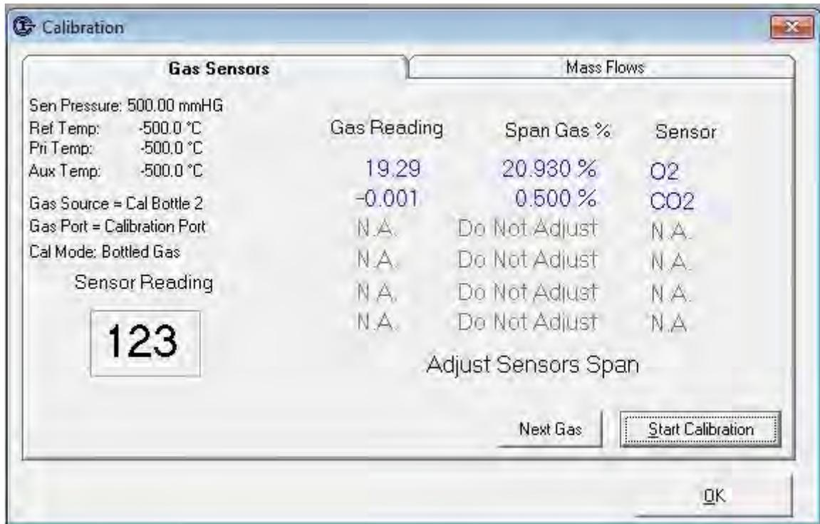
Press next gas and repeat the previous 2 step again for each cylinder (gas bottle) until all gas sensors have been calibrated. After the last cylinder the software will prompt you to turn off the calibration gas bottle.
