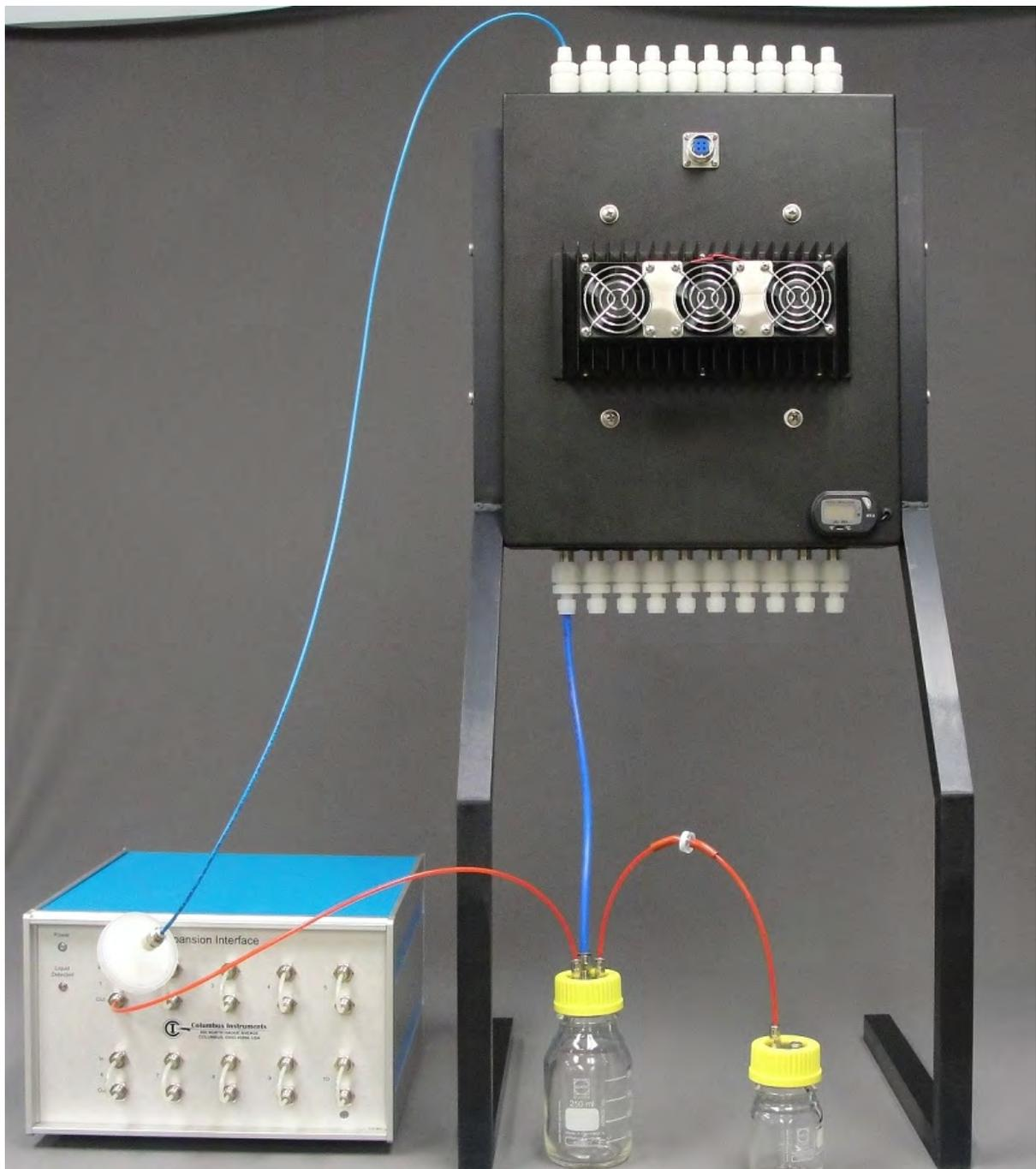
Connection with condenser with 2 port flask
