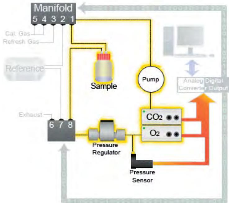
Step 8: After we measure the head space of the first sample, the gas sensors are purged to remove any residual sample gas.. This is necessary in order to prevent the previous sample's readings to interfere with the next, and to prevent them from mixing back into the next sample's head space.
