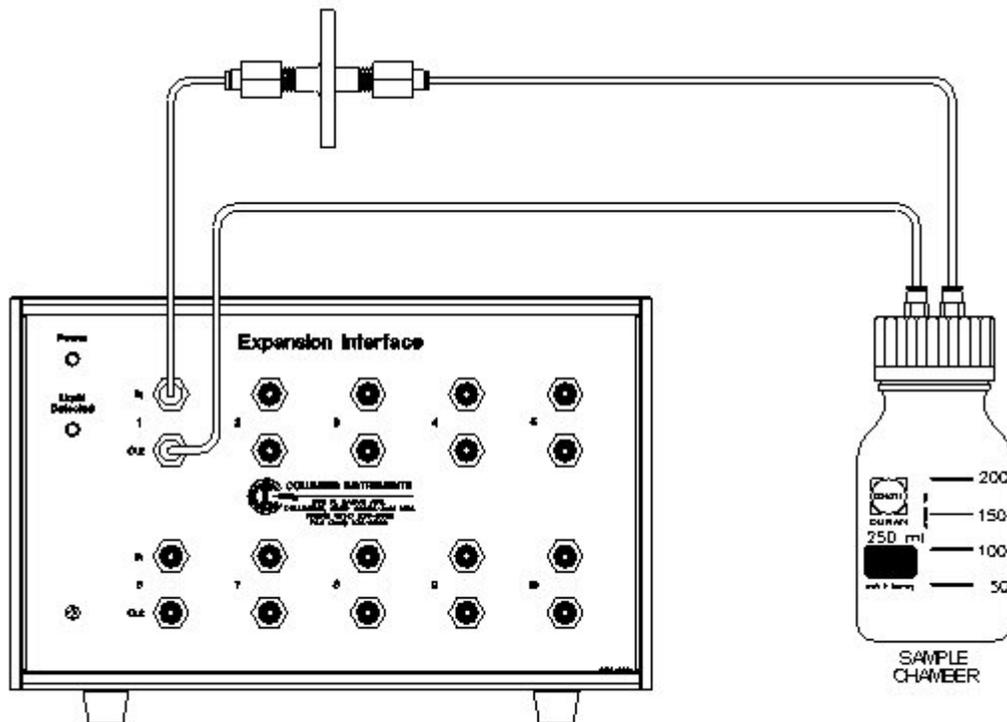
**\* NOTE: This circuit detects liquid by measuring conductance, it will not work with distilled water.**
